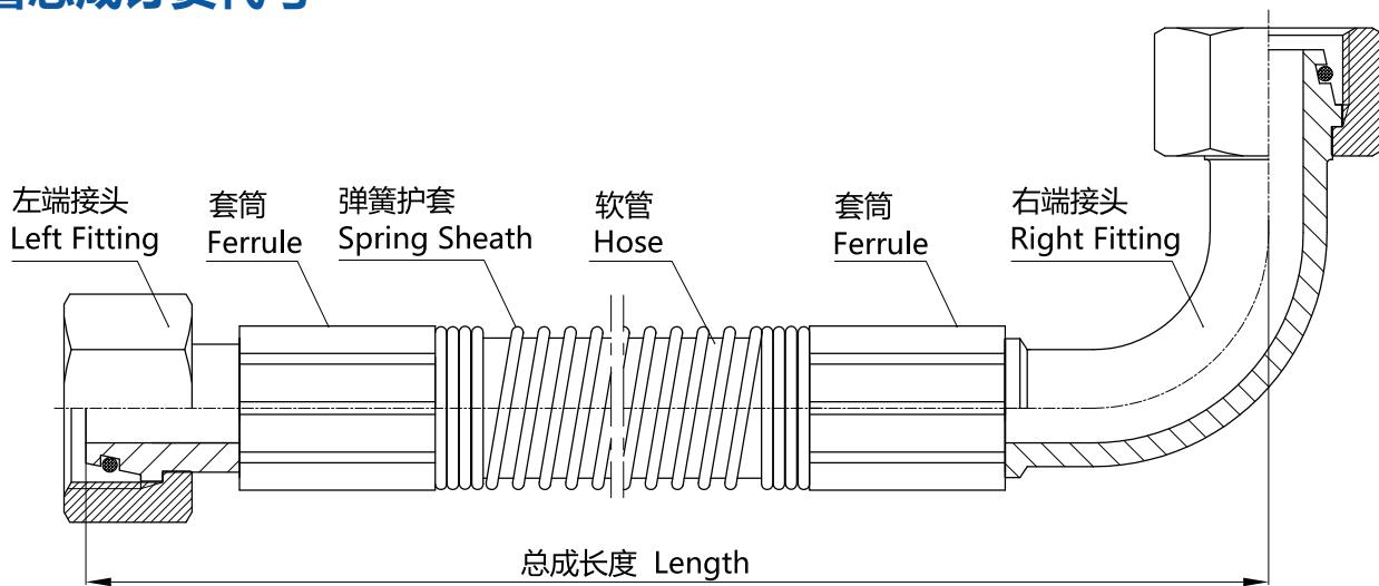
如上图示，液压软管总成由软管、左端接头、右端接头、套筒扣压而成。左端接头与右端接头形状或类型可以相同，也可以不同；护套可以不用或采用其他类别的护套。As shown in the figure above, the hydraulic hose assembly consists of a hose, a left-end fitting, a right-end fitting, and a crimped ferrule. The left-end and right-end fittings can be of the same type or different types; the protective sleeve may be omitted or replaced with another type of sleeve.
